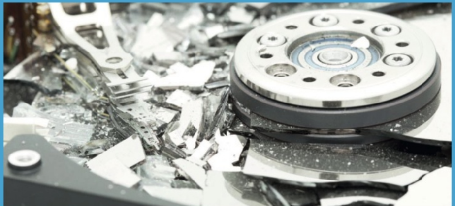
▲ Some hard-drive platters are made of glass. Try not to drop those ones.
